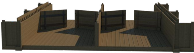
Digital model for use in low-resolution water defence prototype of double sluice at Northeye with top timbers removed
